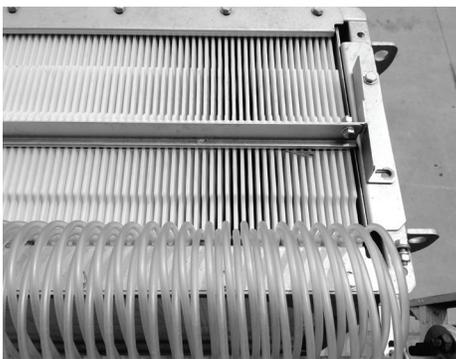
Membrane Bioreactors provide superior effluent quality that can meet the most stringent effluent criteria in North America through the use of a conventional activated sludge process combined with membrane filtration for solids separation. The membrane filters have tiny pores eliminating solids in the effluent and providing superior treatment. The high mixed-liquor suspended solids in our MBR allows for minimized plant footprint and sludge production rates.
