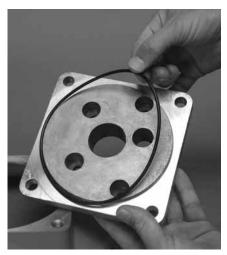
Next, remove the center block adapter plate o-ring and inspect for nicks, gouges, chemical attack or abrasive wear.
