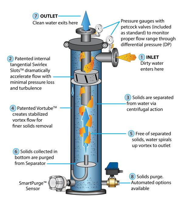
LAKOS eJPX Separators feature improved internals and increased efficiencies as compared to our JPX Separators. To learn more about how our JPX Separators operate, see LAKOS Literature LS-631 & LS-632.
