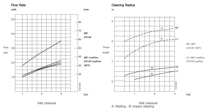
For Clip-on models, the flow rate is increased by approx. 0.2 m<sup>3</sup>/h
