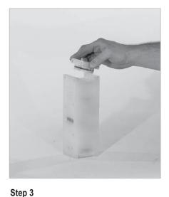
Remove air valve end cap to expose the large end of the air valve spool by lifting up on the air valve end cap once the bolts have been removed.
