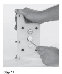
Inspect the center block shaft and air control spool Glyd™ rings (4) for wear. If replacement is necessary, use an O-ring pick to remove the used Glyd™ rings then replace with genuine Wilden replacement parts.
