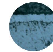
Bending test: Ductile hard chrome coating Result: Excellent adhesion to the basic material, without cracks.
