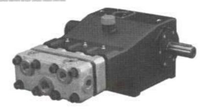
HD Series Triplex Plunger Pump with solid shaft. Cast iron pump body with nickel-treated cast iron head. Crankshaft is nitrided, hardened and tempered alloy steel. Forged steel connecting rods with anti-friction bearings. Solid ceramic plungers.
