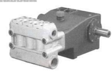
KL Series Triplex Plunger Pump with solid shaft. Cast iron pump body with nickel-treated cast iron head. Crankshaft is nitrided, hardened and tempered alloy steel. Forged steel connecting rods with anti-friction bearings. Solid ceramic plungers.
