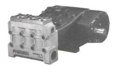
MS Series Triplex Plunger Pump with gear box. Cast iron pump body with nickel-treated cast iron head. Crankshaft is nitrided, hardened and tempered alloy steel. Forged steel connecting rods with anti-friction bearings. Solid ceramic plungers.
