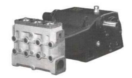
LH Series Triplex Plunger Pump with gear box. Cast iron pump body with nickel-treated cast iron head. Crankshaft is nitrided, hardened and tempered alloy steel. Forged steel connecting rods with anti-friction bearings. Solid ceramic plungers. Specify RPM.
