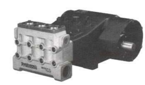
MH Series Triplex Plunger Pump with gear box. Cast iron pump body with nickel-treated cast iron head. Crankshaft is nitrided, hardened and tempered alloy steel. Forged steel connecting rods with anti-friction bearings. Solid ceramic plungers. Specify RPM.
