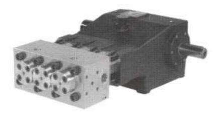
VH Series Triplex Plunger Pump with solid shaft. Cast iron pump body with special steel head. Crankshaft is nitrided, hardened and tempered alloy steel. Forged steel connecting rods with anti-friction bearings. Solid ceramic plungers.
