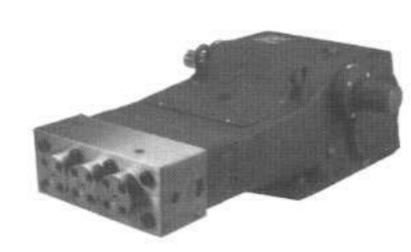
SH Series Triplex Plunger Pump with gear box. Cast iron pump body with stainless steel head. Crankshaft is nitrided, hardened and tempered alloy steel. Forged steel connecting rods with anti-friction bearings. Solid ceramic plungers. Specify RPM.
