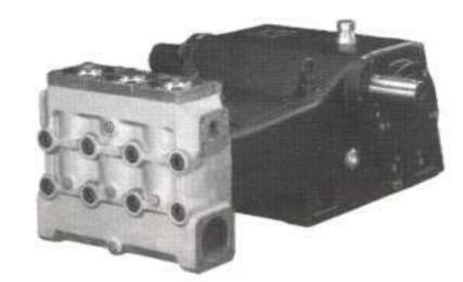
LHZ Series Triplex Plunger Pump with gear box, 316 stainless steel manifold and wetted parts (including valve plate and seat). Ideal for reverse osmosis, ultra- filtration, chemical and water treatment, sea water blasting applications. Specify RPM.
