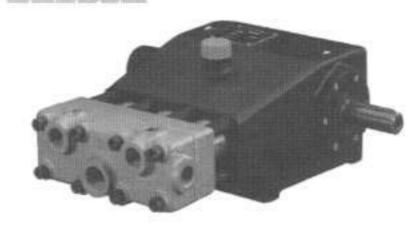
EK Series Triplex Plunger Pump with solid shaft. Cast iron pump body with nickel-treated cast iron head. Crankshaft is nitrided, hardened and tempered alloy steel. Forged steel connecting rods with anti-friction bearings. Solid ceramic plungers.
