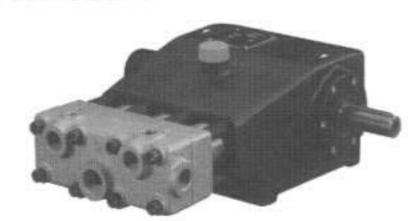
EKLN Series Triplex Plunger Pump with solid shaft. 316 stainless steel manifold and wetted parts; 431 stainless steel valve plate and seat. Ideal for reverse osmosis, ultra-filtration as well as chemical and water treatment applications.
