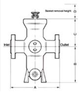
High Pressure Gas Filters – Simplex J Type 2" - 10" (50mm - 250mm)
