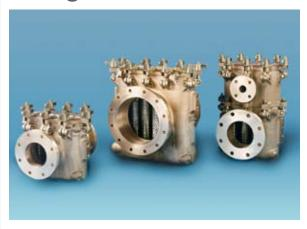
Normally supplied in Gunmetal or Aluminium Bronze with a Cupro-Nickel screen, it is suitable for low or medium pressure applications such as sea water cooling, fire fighting applications, hydraulic and fuel oils and product transfer. The Plenty Seaguard is ideally suited for shock and non magnetic service.
