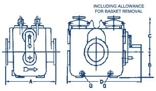
Changeover gear on right hand side looking on inlet as standard. Available on left hand side as optional alternative at extra cost.
