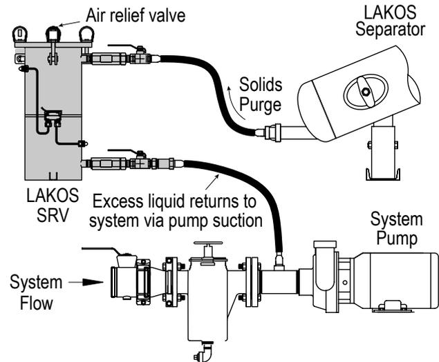
Separated solids are purged at a continuous rate directly into a solids recovery vessel, which is integrally equipped with a solids collection bag in a stainless steel basket.
