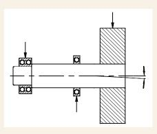
Cantilevered designs and resulting shaft deflection
