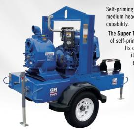
Self-priming centrifugal, heavy-duty solids-handling, medium head, engine driven pumps with reprime capability.
