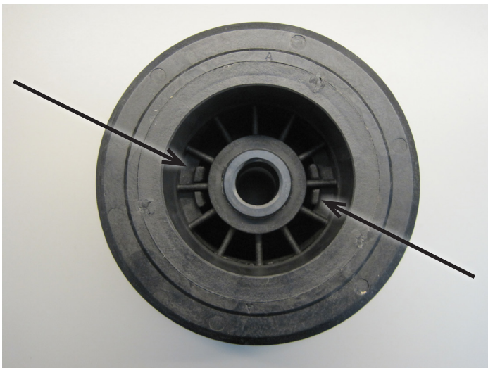
Single Piece Impeller drive hub w/snap-fit prongs
