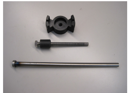
figure 1A: Impeller Removal Tool includes: prong release tool, 5" long bolt, bushing, & drive pin.
