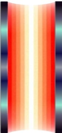
Disc pumps employ the principles of boundary-layer adhesion and viscous drag, which produce pulsation-free, laminar flow.
