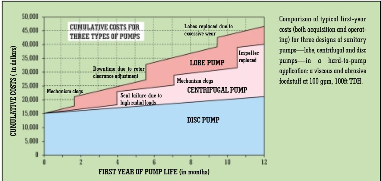
Comparison of typical first-year costs (both acquisition and operating) for three designs of sanitary pumps—lobe, centrifugal and disc pumps—in a hard-to-pump application: a viscous and abrasive foodstuff at 100 gpm, 100ft TDH.
