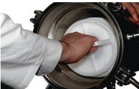
'Twist-to-lock' cartridge seating mechanism
