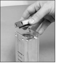
Step 5 Remove air valve end cap to expose air valve spool.
