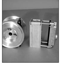
Step 2 Remove the air valve and muffler plate from the center section.
