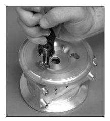
Step 7 Remove pilot spool retaining snap-ring on both sides of center section with snap-ring pliers.
