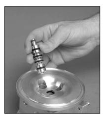
Step 8 Remove pilot spool assembly from center section.
