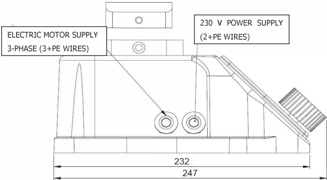
Figure 4 Side view of the supply lines
