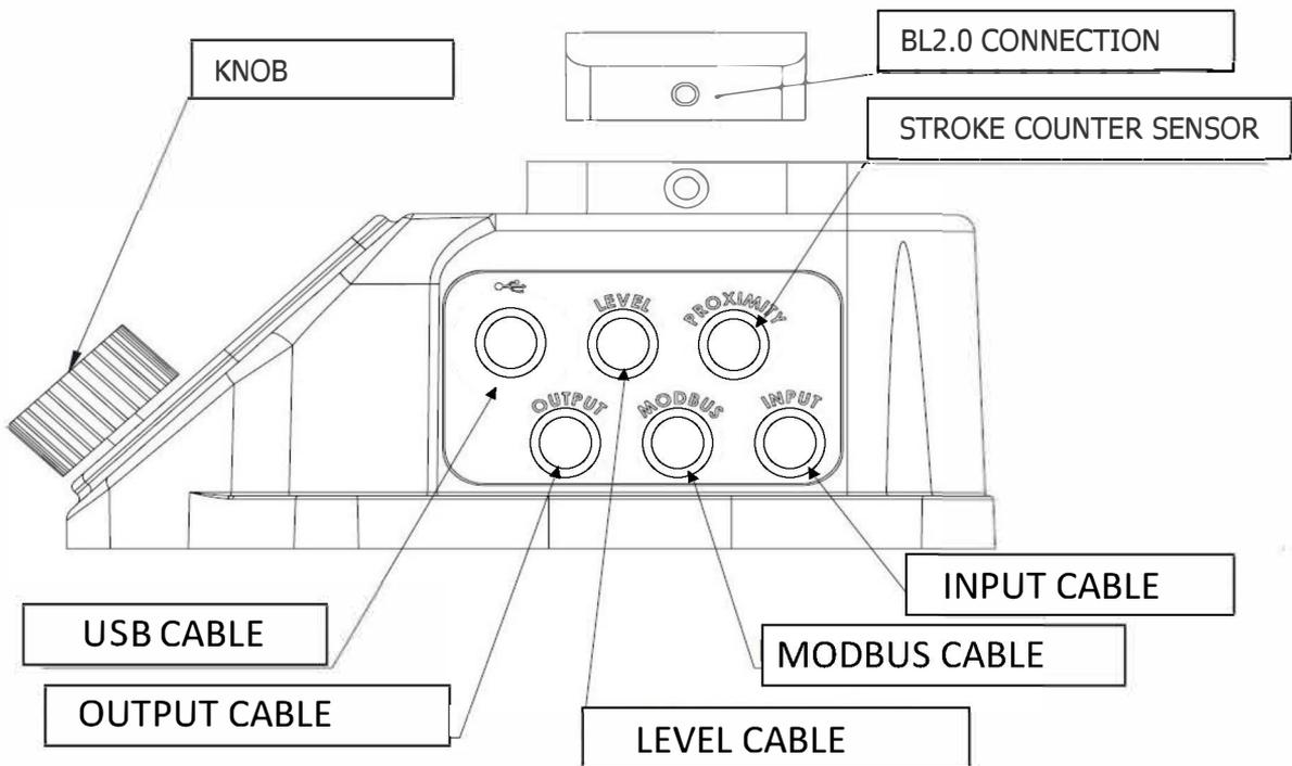
Figure 5 Side view of the supply lines
