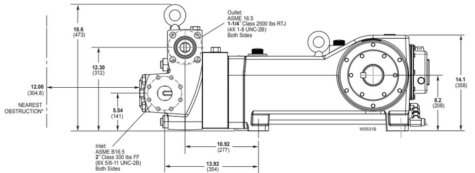
\*Contact factory for obstruction distances closer than 12 inches (304.8 mm).
