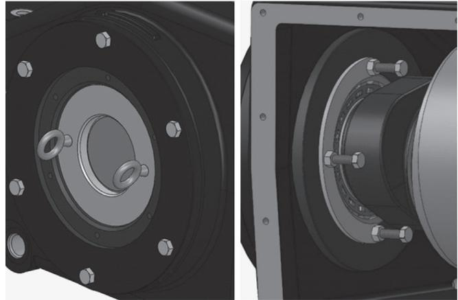
**Crankshaft Alignment Donut      Crankshaft Installation Bar**
