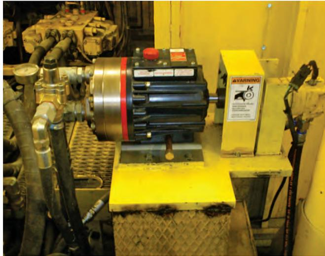
*Hydra-Cell providing dust control on a rotary drilling machine.*
