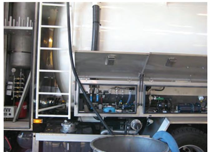
Hydra-Cell used for pumping liquid explosives into an injection rig.
