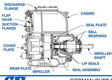
Shown with Optional Suction & Discharge Spool Flanges (Available in ASA or DIN Standard Sizes).
