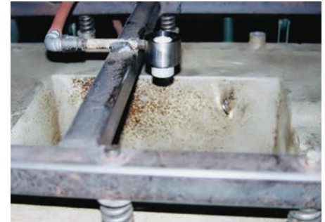
A Model 121021 1-1/4" (32mm) High Temperature Air Amplifier directs hot air to a rotational mold cavity for uniform wall thickness of the plastic part.
