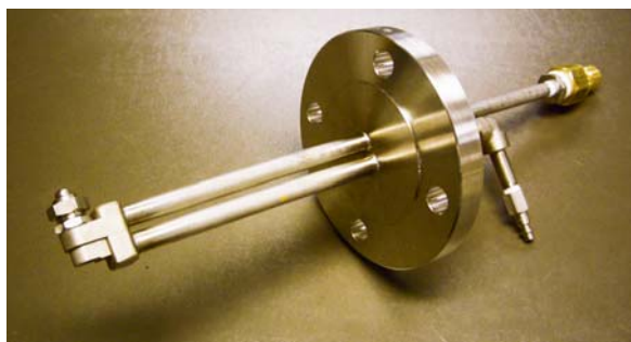
Spray lance (see page 107) with a right angle XA and quick-connect fittings
