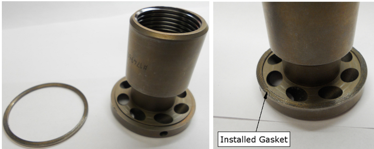
Assembly 5: Install Spillback Gasket
