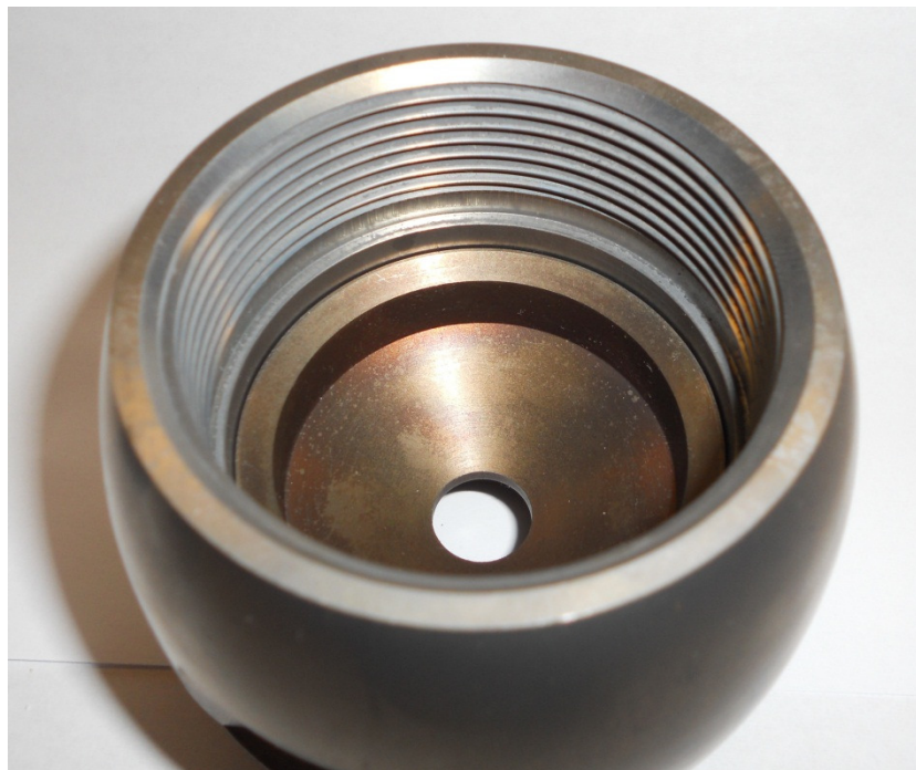
Assembly 9: Install Fluid Cap into Cap Nut
