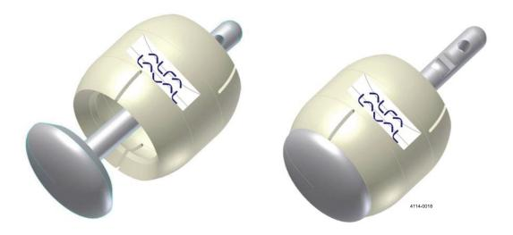
2. The cylindrical end of the stator (3) is then inserted into the centre hole of the Connector (1). The stator can be inserted to its full extent in one position only. When the stator is fully inserted into the connector, the rotor (2) will be fixed between the bearing surface of the stator and connector
