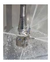
The new Alfa Laval BurstClean+ tank cleaning process uses the rotary spray head concept to soften stubborn residues, followed by the impingement technology of a rotary jet head to quickly remove those residues.
