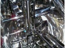
Personal care industry: toothpaste tank after 6 minutes of rotary jet head wash cycle.
